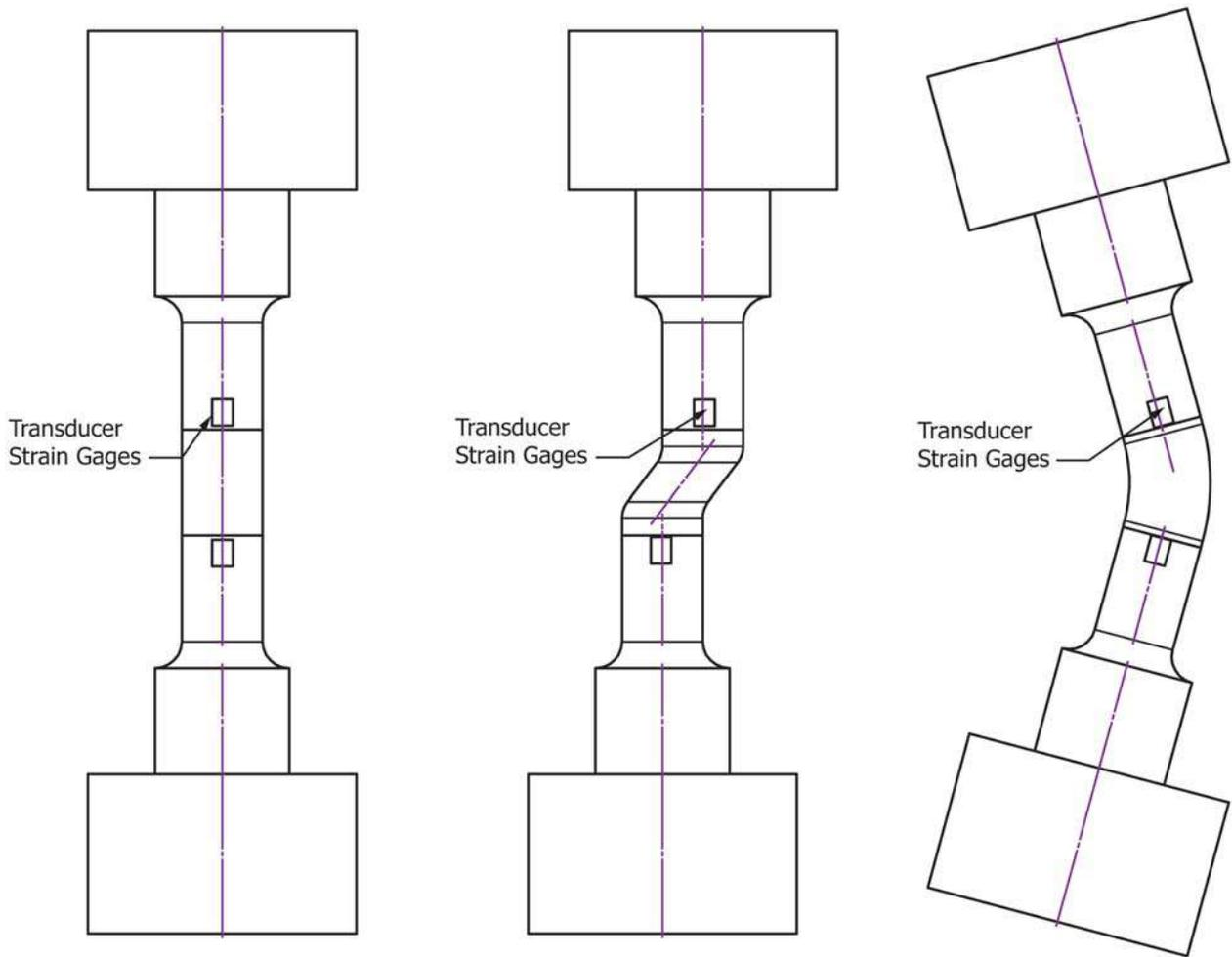
**FIG. 6 Illustration of Strain-Gaged Alignment transducer**
