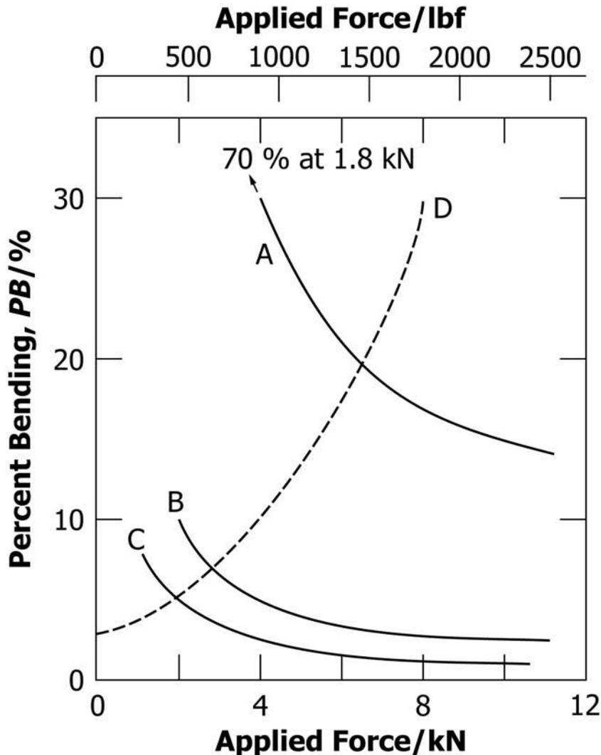
NOTE 1—Curve A: Machine 1, threaded grip ends (1)
