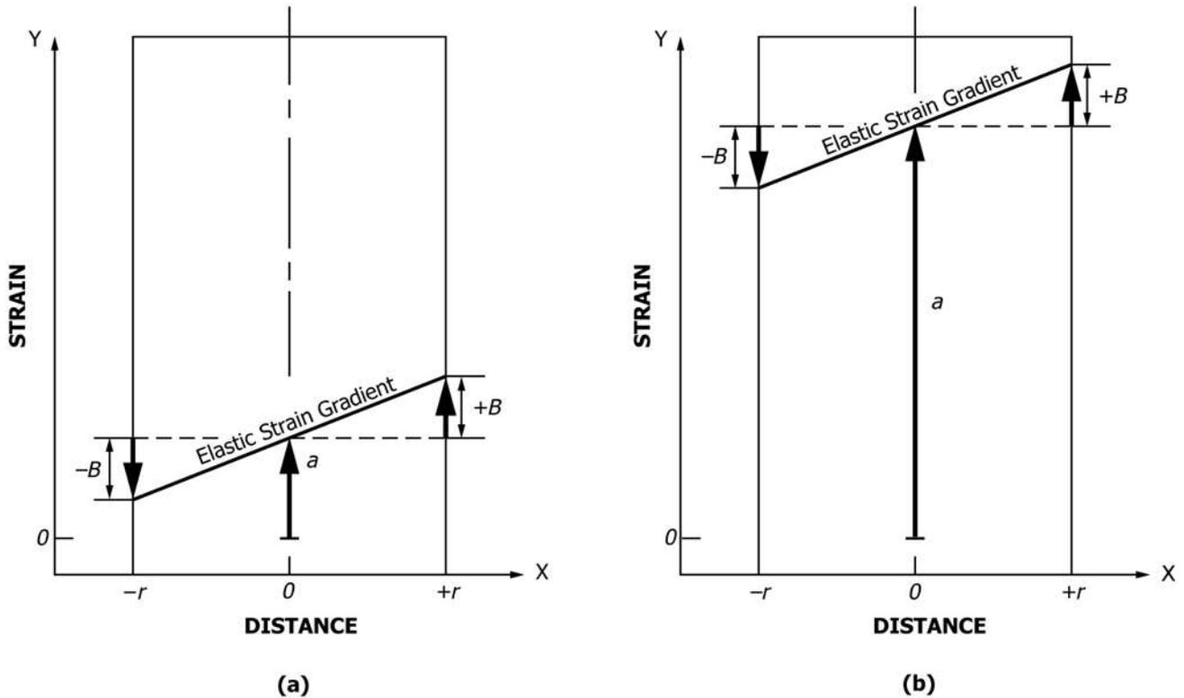
NOTE 1—A bending strain,  $\pm B$ , is superimposed on the axial strain,  $a$ , for low-axial strain (or stress) in (a) and high-axial strain (or stress) in (b). For the same bending strain  $\pm B$ , a high-percent bending is indicated in (a) and a low-percent bending is indicated in (b).
